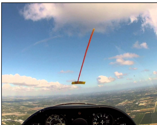
Figure 18-7. A string attached to the windshield of gyroplane is often used to indicate rotation about the yaw axis. An inclinometer may also be used.
