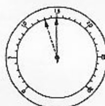
8. LEAKY VALVE Regular drop about 2 inches.
