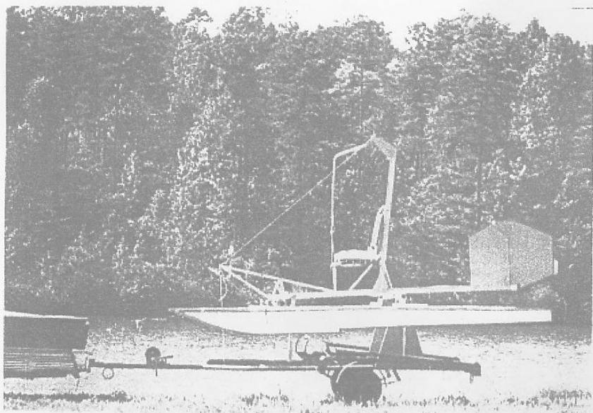
FLOAT INSTALLATION. From left to right and from top to bottom: 1. Rear Axle attachment; 2. Front Axle attachment, note inspection hole covers; 3. Gyro on floats ready for flight test, transported on a small boat trailer; 4. First test hop close to the water, in towed flight.
