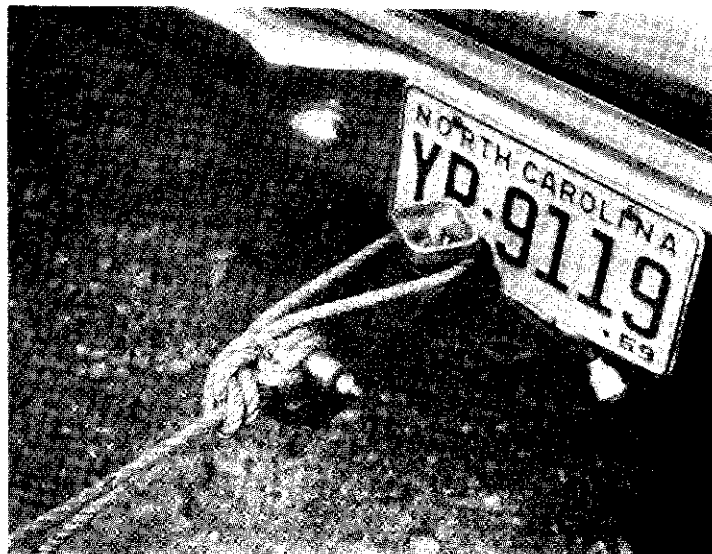
Fig. 13—A closeup of the approved tow hitch and the rope fastening. It is important that the tension end of the rope go directly over the solid bar without kinks or knots.
